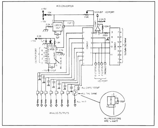
Fig. 8-4. A schematic diagram of the A/D converter.
